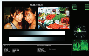
Waveform + Vector Scope + VPID SDI-1, Waveform / Vectorscope, 16 CH Audio Level Meter, VPID & Time Code
