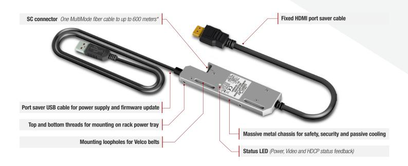
The HDMI20-OPTJ-TX90 and HDMI20-OPTJ-RX90 are HDMI 2.0 compatible optical fiber extenders. These units transfer uncompressed HDMI 2.0 class signals with embedded audio to up top 600\* m distance, over one MultiMode fiber cable. Embedded HDMI audio signals include Dolby TrueHD and DTS-HD Master Audio.
